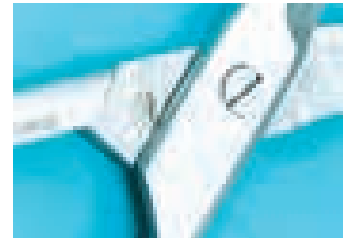
Joint showing wear due to inadequate lubrication
